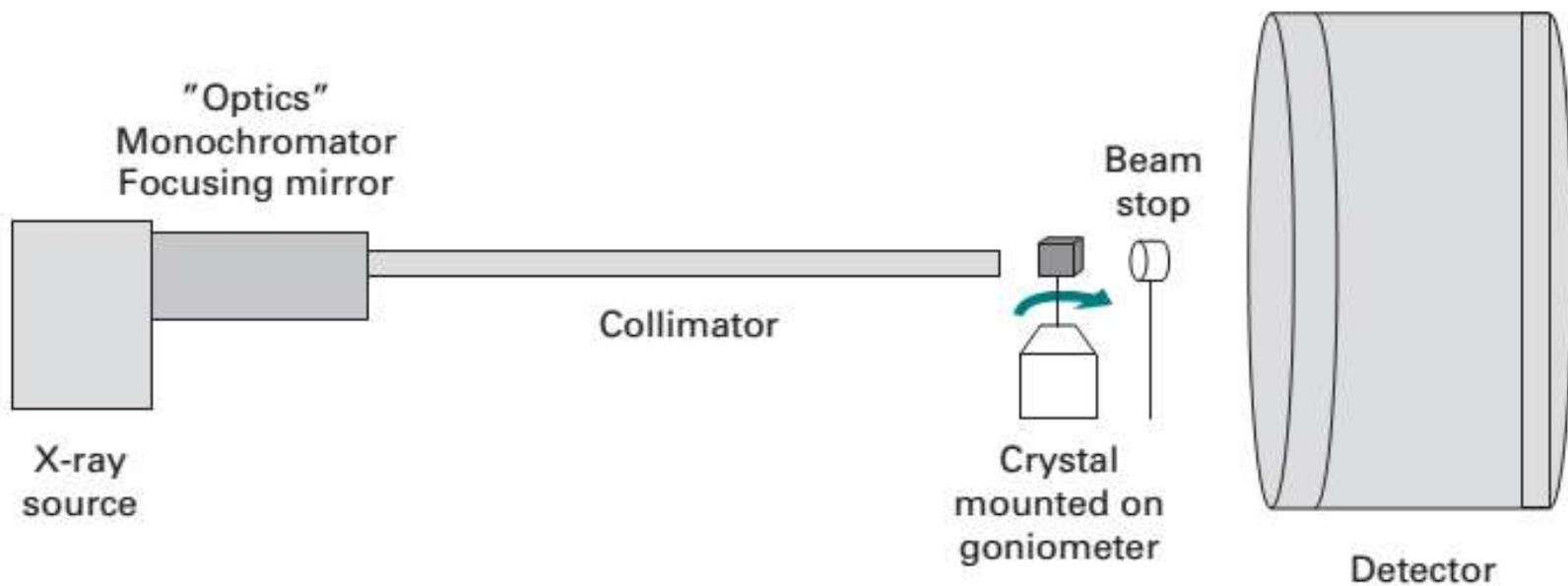
Instrumentation for X-ray diffraction. The most common X-ray sources are (a) particle storage rings which produce synchrotron radiation, and (b) rotating anode tubes. The schematics of an X-ray diffractometer are shown in (c).
